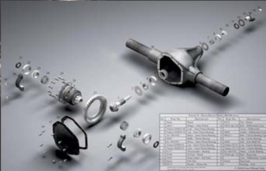
Feature-based CAD constructs designs from smaller, interdependent parts
